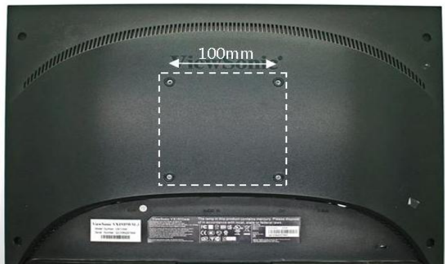
VESA Compatible display with 100mm square screw pattern
